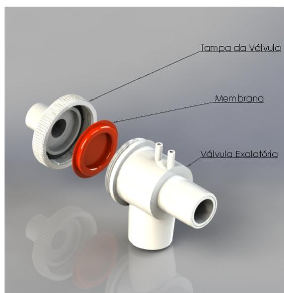
**FIGURA 7: MONTAGEM VÁLVULA EXALATÓRIA**
